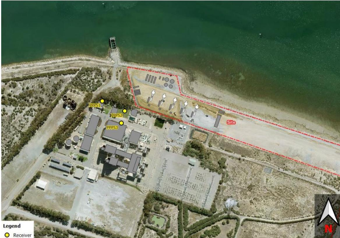
Figure 4.2 Noise Sensitive Locations at the adjacent Pelican Point Power Station (PPPS).
